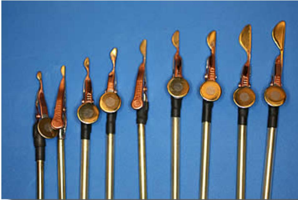
Wing burners in sizes from 22 to 10
