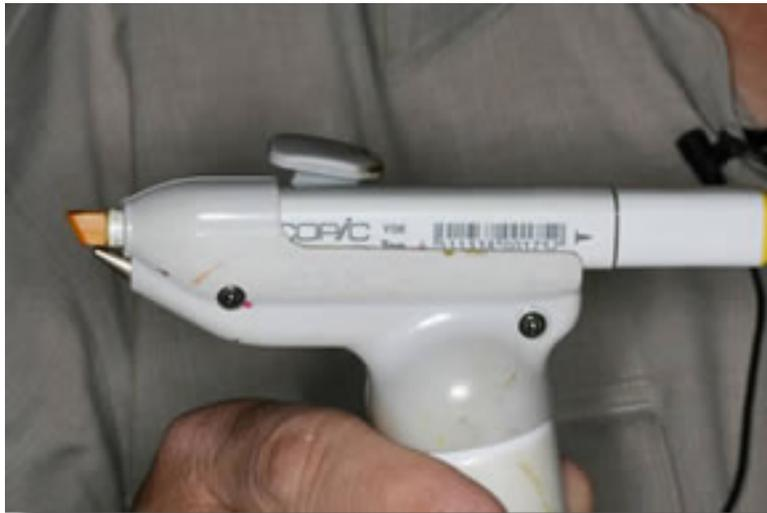
6. The next steps involve painting the fly to look like the baitfish the big fish you want are eating. Randy uses a Copic sprayer and pens. It is more convenient than an air brush. The sprayer needs a source of 50 psi compressed air. This might come from compressed air cans or a compressor. Some tying instructions I found on the internet recommended waterproof pens to color the flies. The results were simple light belly and grading darker on the back.
